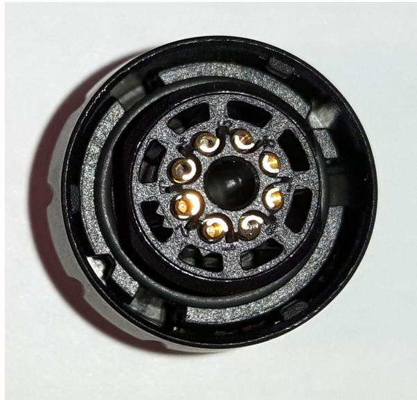
View from the back of the cable connector, to help allocate PIN 1 is marked with 1 arrow, PIN 2 is marked with 2 arrows in a clockwise direction.
